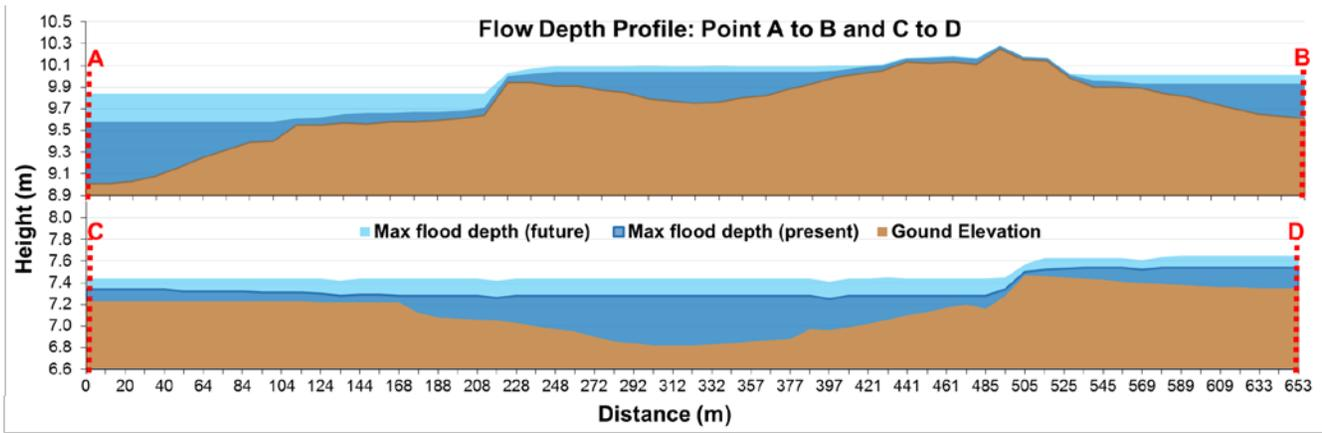
Appendix B. Baseline and near future flow depth profile, locations (A, B, C, and D) can refer to Fig. 8 and Fig. 9.
