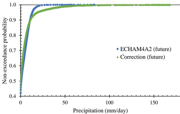
Fig. 5. Simulated and corrected CDF of daily precipitation in the near future (2030s)
